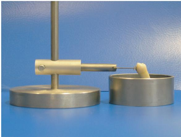
**Fig 1.** Specimen oriented with guiding device into ring.
